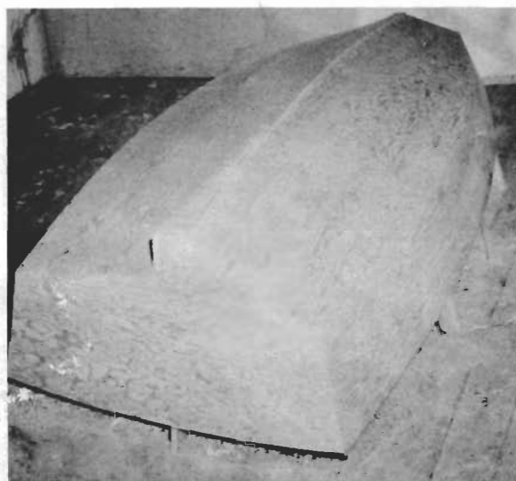
Bottom trimmed — skeg in place.
