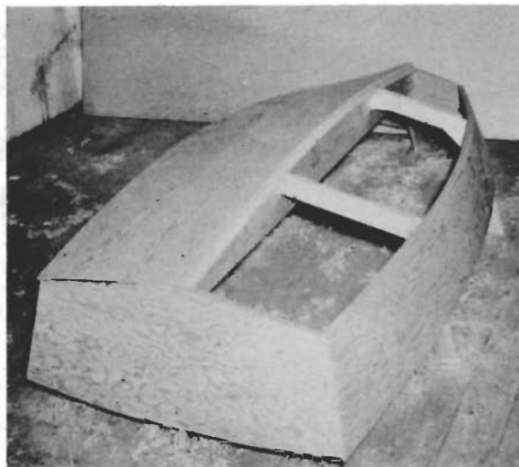
First bottom in place.
