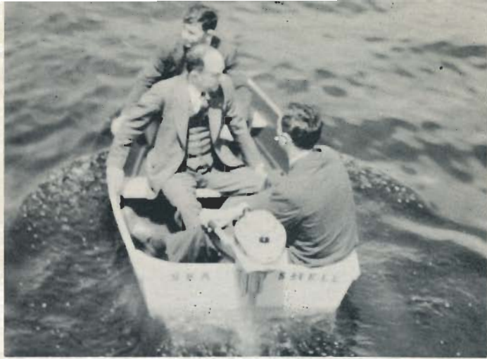
OUTBOARD —The smallest outboard pushes her with ease. Her slanting bow transom keeps her "head up" in rough going.
