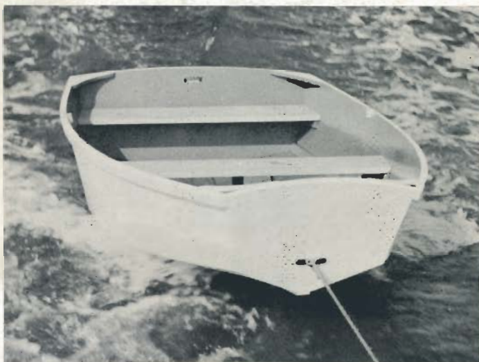
TOWING —Because of her "V" bottom and light displacement she tows without yawing and is light on the painter.
