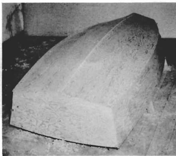
Bottom complete — ready for trimming.
